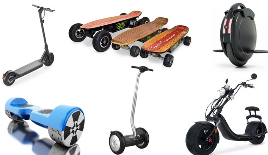
Fig. 1. Various types of electrically powered single-person vehicles, from top left: electric scooter, different types of e-skateboards, airwheel, hoverboard, Segway, and fat glider.
